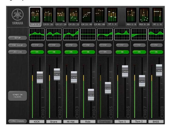
Across the top of the screen, all Input, Mix and Matrix level meters and faders are displayed in blocks of eight. This is the "Navigation/Meter Bridge". Press any of these blocks to select which channels are viewed in the fader strips below.
