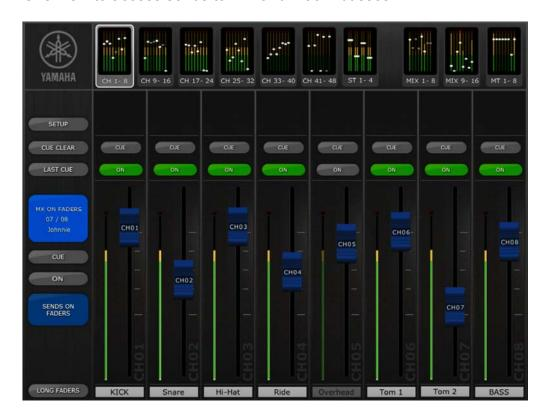
A large button will appear to show the currently selected Mix or Matrix, and its name. The colour of this button matches those used on the M7CL console. [CUE] and [ON] buttons appear below, allowing the currently active Mix or Matrix bus to be Cued and turned On/Off.
